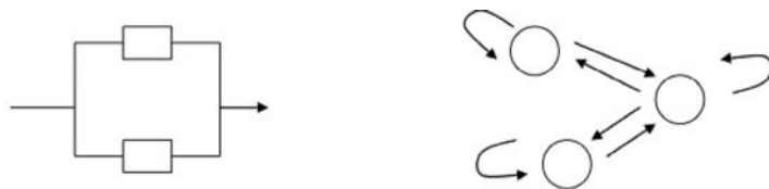
Figure 1. Parallel system of two identical units: (a) block diagram; (b) state diagram.
