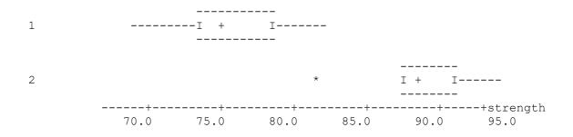
The above boxplots signal that there are differences in the tensile strengths of the two (manufacturers) groups, which is also clearly apparent in the scatter plot below. We need to explore further this manufacturer's difference:
