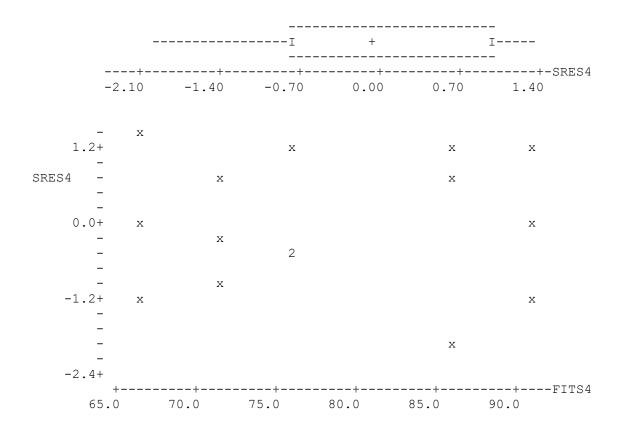
Since we accept as valid the regression model results, it means that we do not have enough grounds to reject the null hypothesis. Hence the regression of tensile strength on thickness, for both manufacturers, does not differ either in level or in rate or in both.
