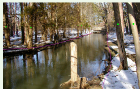
Fig. 8. Visual estimation of bankfull conditions and required water depth to entrain (suspend and move downstream) sediment at site F in the Waterworks reach. Pink lines represent bankfull conditions while green dots on trees mark the approximate water height necessary to entrain the bed material at this location.
