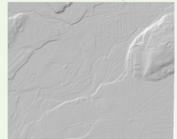
Fig. 12. The Waterworks Reach of Otter Creek was classified according to the Rosgen system as having the morphology (appearance) of a braided stream. This is supported by this hillshade LIDAR image that shows braid features in the Waterworks reach that contrast with the channelized reaches of Otter Creek elsewhere. However, Otter Creek today is not an active braided stream. Rather, it is a relic of the Valley Heads re-advance, and it has remained virtually unchanged by water flow for ~14,000 years.
