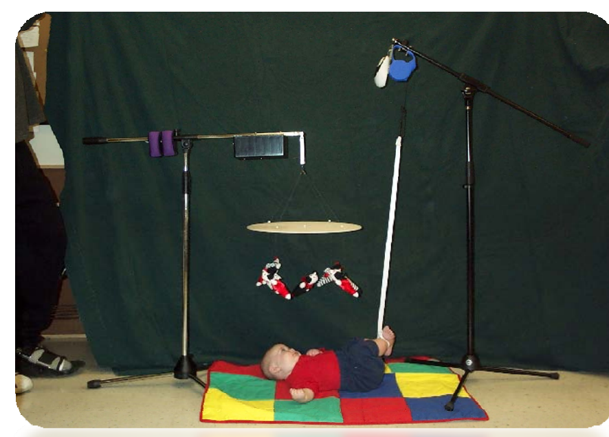
A computerized apparatus, analogous to Rovee-Collier's (1969) mobile procedure, measured kicks and controlled presentation of reinforcement (movement of the mobile).
