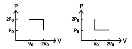
1) In the first process the gas expands isobarically, then is reduced to half the pressure isovolumetrically.
