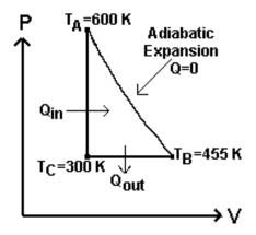
$$\begin{aligned} Q_{in} &= nC_V \Delta T = (1) \left(\frac{3}{2}8.314\right) (600 - 300) = 3741 \text{ J} \\ Q_{out} &= nC_P \Delta T = (1) \left(\frac{5}{2}8.314\right) (300 - 455) = -3222 \text{ J} \\ e &= 1 - \frac{\left|Q_{out}\right|}{Q_{out}} = 1 - \frac{3222}{3741} = 14 \text{ the efficiency of the cyclic process.} \end{aligned}$$
